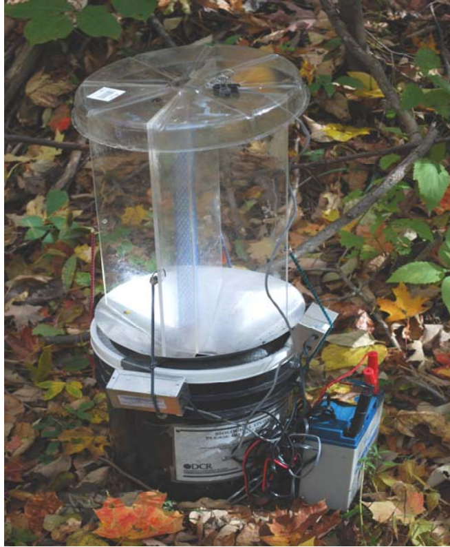
Ultraviolet light trap used for invertebrate sampling at Powell Mountain Karst Preserve, Wise County, Virginia
